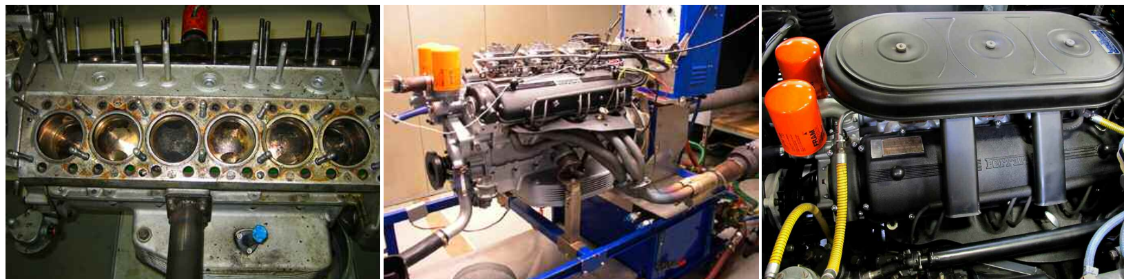
ABOVE, LEFT TO RIGHT Original V12 engine was smoking during acceleration, so Virtuoso rebuilt it with proprietary cams and pistons; engine dyno was used to tune the triple Weber carburetors; restored engine bay looks factory original, with a hint of patina.
