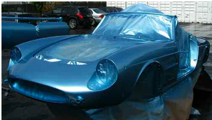
ABOVE LEFT 330 GTS's nose required a few repairs. BELOW Environmentally friendly water-based paint mimics the hue of original lacquer finish.
