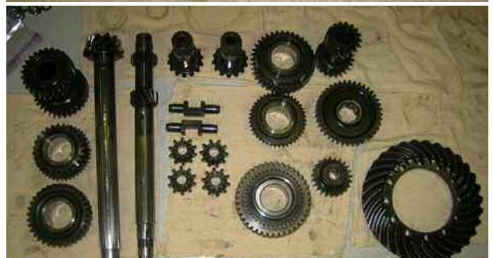
BELOW RIGHT Transaxle was broken down for inspection, and its internal components were sent out to be crack-checked.
